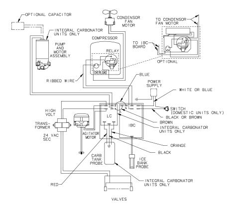
**FIGURE 9. WIRING DIAGRAM**
